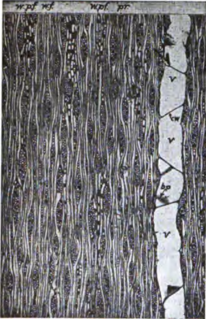
FIG. 5. — Tangential Section of Circassian Walnut. (Cir. 212, U. S. For. Ser.)
